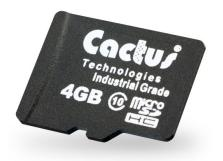
**The Cactus Technologies Secure Digital microSD Card (SD) - 803M Series** is a low capacity solid-state flash memory product that complies with the Secutre Digital Card Association (SDA) standard. Cactus microSD Cards provide up to 4GB (Class 6) of formatted storage capacity and are designed to be used in applications which require reliable, high performance solid state storage in a small form factor.
