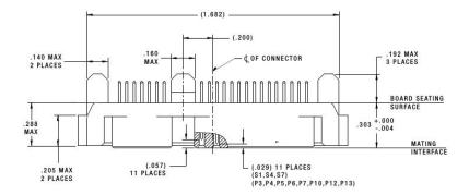
Below are some details about this connector: Device connector part number: RS2-PRCE22-X
