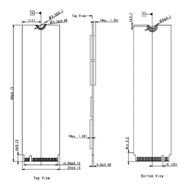
Note: the top side thickness is without the heat spreader. Heat spreader adds approximately 0.4mm to the thickness.
