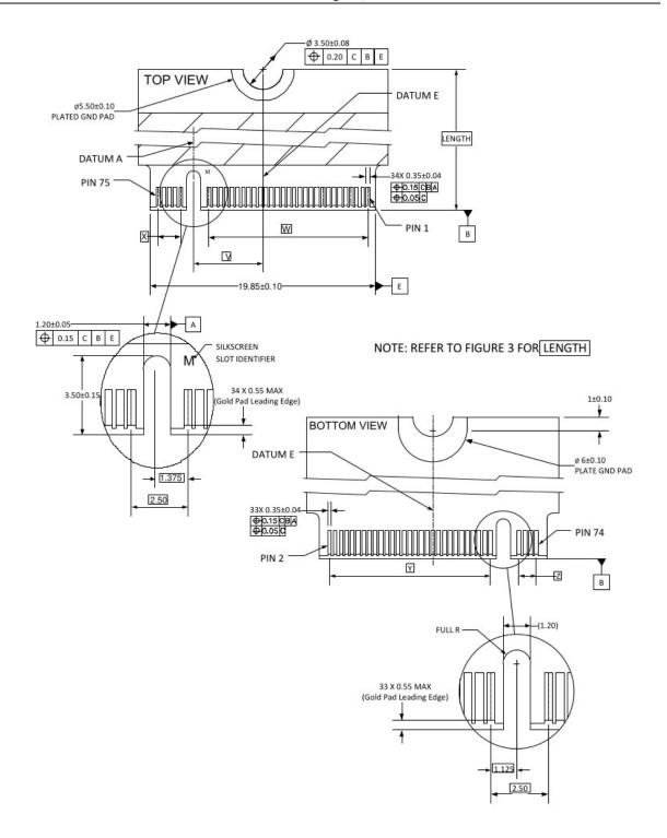
Note: the top side thickness is without the heat spreader. Heat spreader adds approximately 0.4mm to the thickness.
