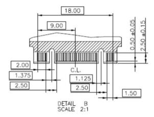
Note: the top side thickness is without the heat spreader. Heat spreader adds approximately 0.4mm to the thickness.
