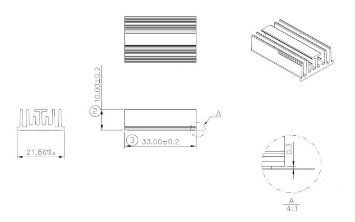
2-2. M.2 2242 SSD Heat Sink Dimensions (for extended temp. version)
