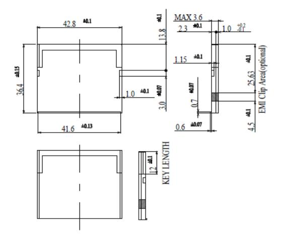
Figure 2-1. Type I CFast Card Dimensions
