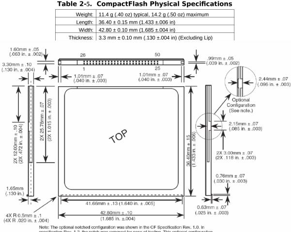
Note: The optional notched configuration was shown in the CF Specification Rev. 1.0. In specification Rev. 1.2, the notch was removed for ease of tooling. This optional configuration can be used but it is not recommended.
