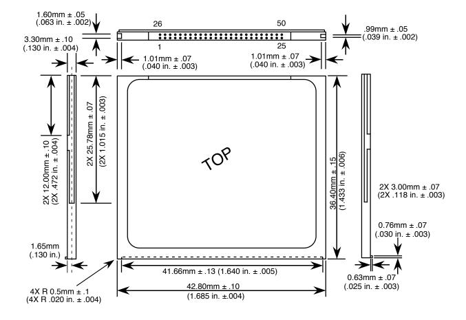
Figure 2-1. CompactFlash Memory Card Dimensions
