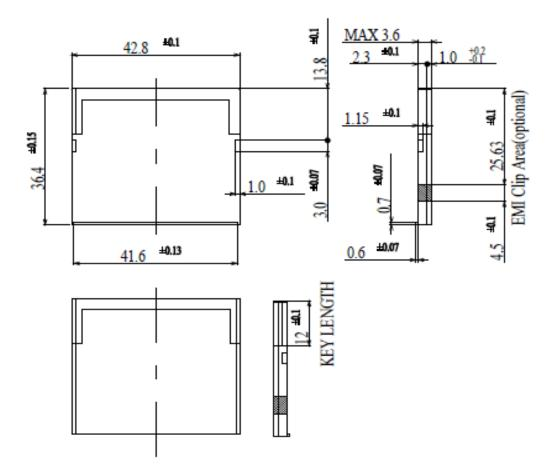
Figure 2-1. Type I CFast Card Dimensions
