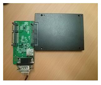
The test fixture has a DC-DC controller and a bus isolation circuit, and is controlled via a serial port connected to a PC. Special test code written by Cactus Technologies<sup>®</sup> randomly shuts off power and isolates the interface bus from the DUT. This ensures that the DUT is not powered via interface bus signals. A typical test sequence is as follows:
