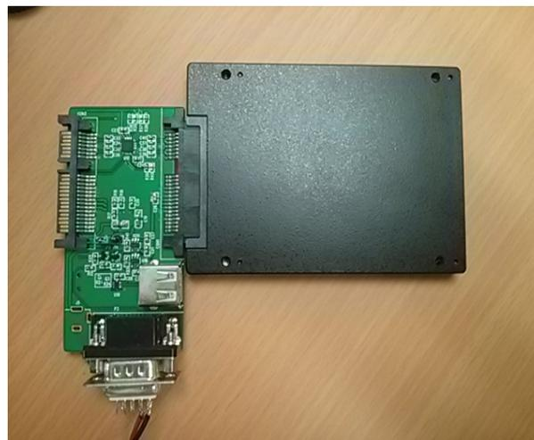
The test fixture has a DC-DC controller and a bus isolation circuit, and is controlled via a serial port connected to a PC. Special test code written by Cactus Technologies® randomly shuts off power and isolates the interface bus from the DUT. This ensures that the DUT is not powered via interface bus signals. A typical test sequence is as follows:
